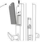
(3) Lift the handle and the lock latch out as normal
