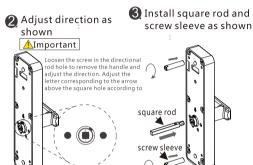
Note: The square rod spring is aligned with the opening in the panel knob sleeve
